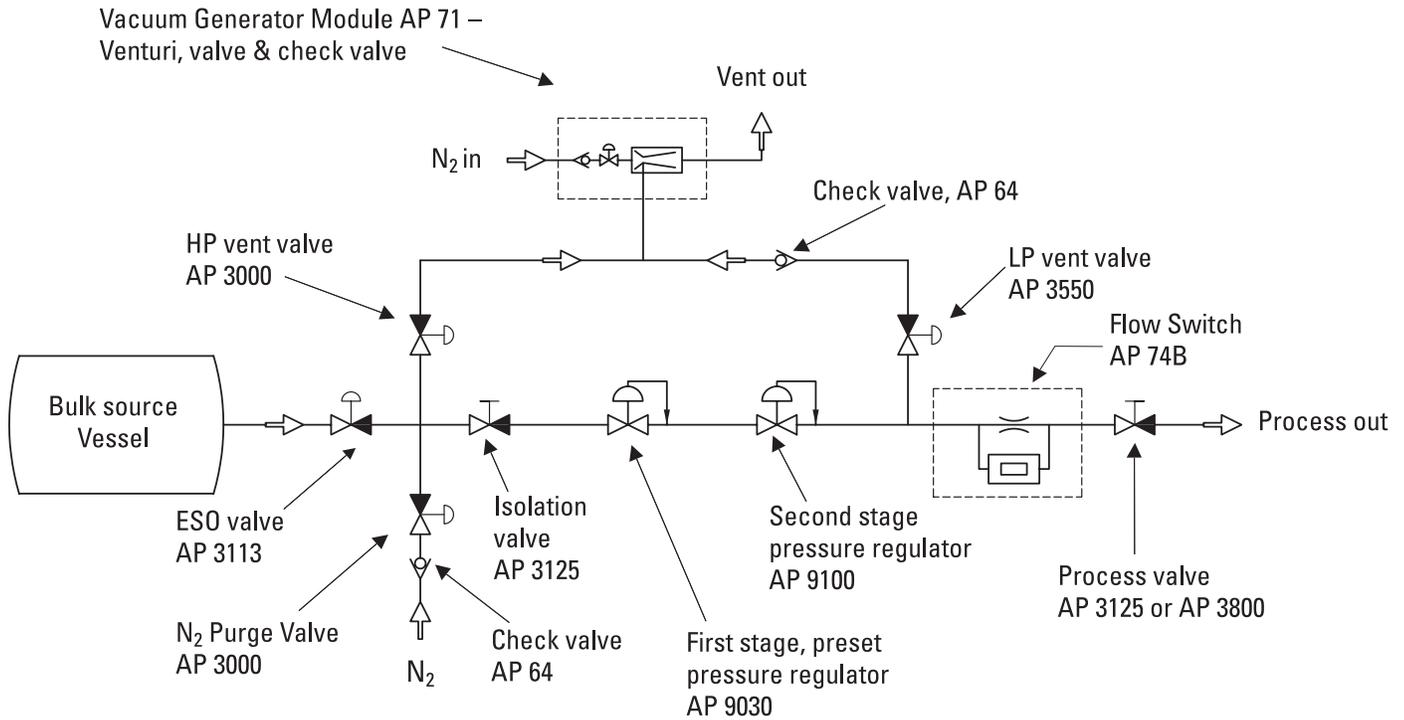
Note: This schematic is intended as an example of AP Tech component usage only. It does not include pressure measurement, filtration, etc. which must be included in a system.
